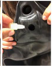
**2.** Once the cap is removed, a transparent safety valve will be visible. The latter must be removed. Help yourself by pushing it from behind or pull it out with another tool
