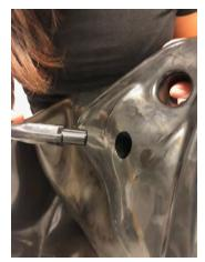
**3.** After removing the valve, insert the nozzle for the hose. The end in the figure must be inserted into the hole, the other into the rubber tube of the water pipe. Add a few drops of bleach to prevent decay of the water inside.
